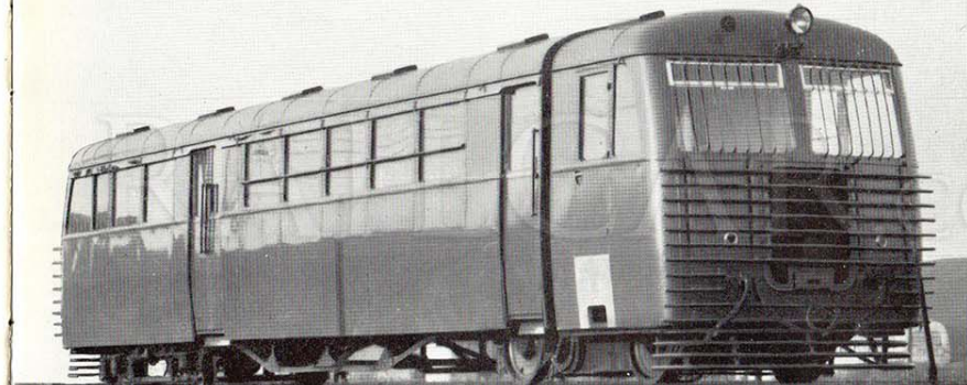
Two of a batch of six railcars for the Paita-Piura coast line Peru. These railcars run inland working in appalling conditions and all the more modern cars have Self-Changing Gearboxes. The frontal grill forms a protection against attacks by Condors and other large birds.
