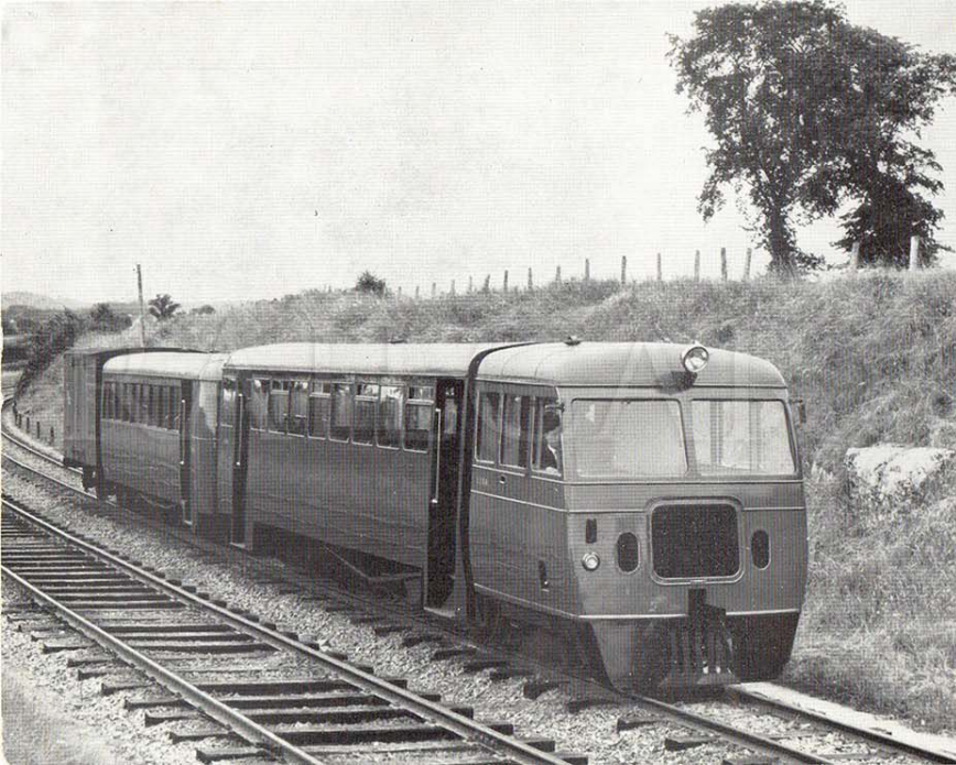
This small railcar used on Irish country routes pulls a trailer and parcel van. The cars are mounted from track level.
